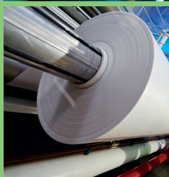
Above and below: Extrusion of ReZorce material at the Zotefoams facility in the Netherlands
