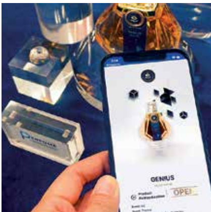
The SIC43NT combines two vital features of tamper detection to verify whether the packaging has been opened and proof of authenticity to ensure the product is genuine.
