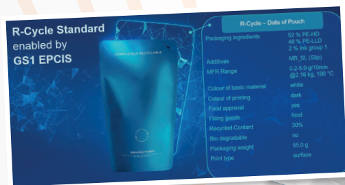
A digital product passport for sustainable plastics, the R-Cycle concept can optimise the recycling process by storing recycling-relevant production data and affixing a clear ID mark on recycled packages
